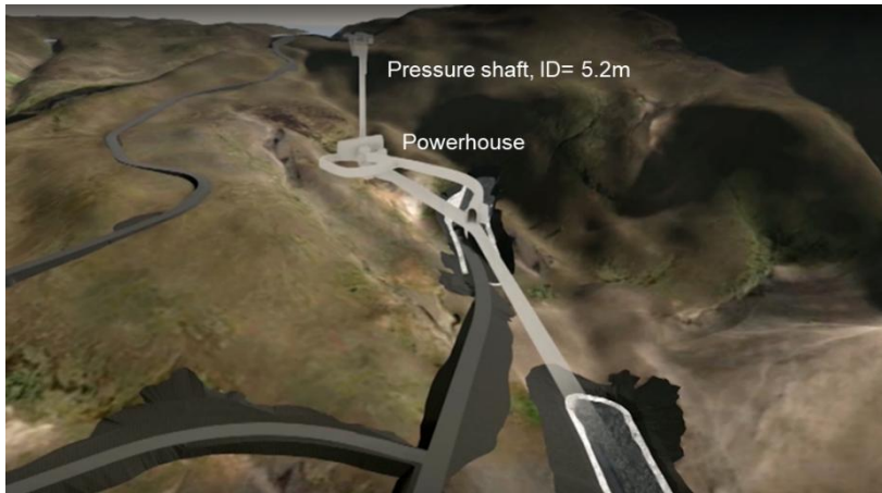
Figure 4. Pressure shaft (steel lined) at Búrfell III excavated by raise bore technology.
