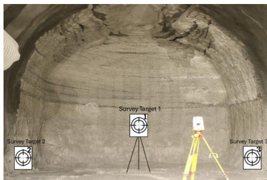
Figure 1. Setup during photogrammetry data collection. Numbered survey targets are placed in the shot to allow orientation of the model
