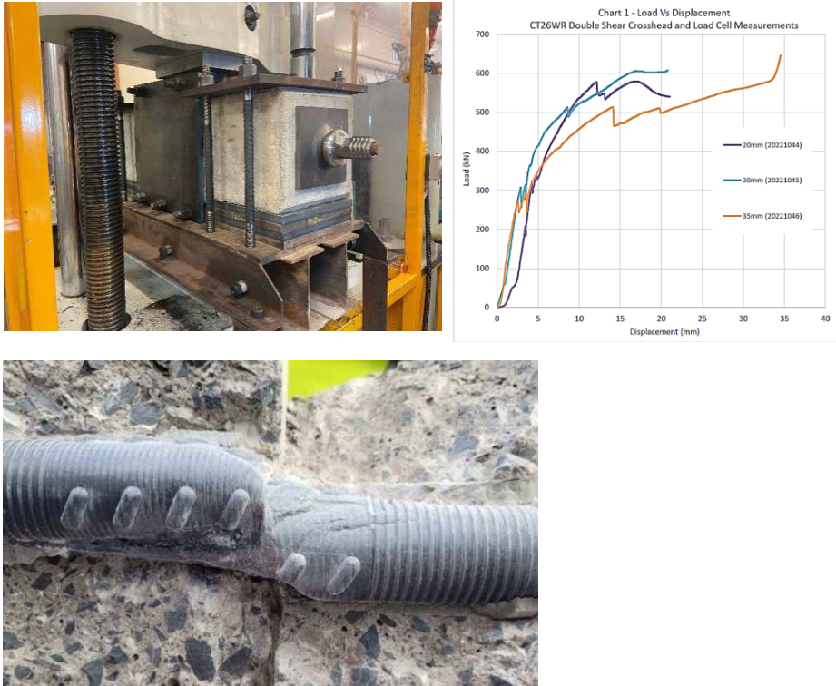
Figure 2. Double shear test of bolt (left); Load-displacement curves of CT26WR double shear tests for 20mm and 35mm limits (right); CT26WR after 35mm shear displacement (bottom)
