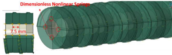
Figure 10. Schematic representation of bond-link elements modeling the rebar–grout interface using four dimensionless nonlinear springs per interval
