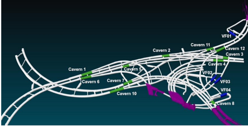
Figure 1. location plan of 11 road caverns (green) and 4 ventilation facilities (blue). Cut-and-cover structures are shown in purple.
