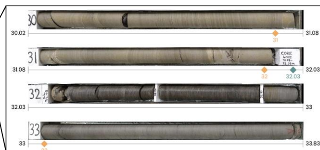
Figure 11. Example of dominant colour extract. Left image: row image composite, middle image: dominant colour representation, right image: close up of row images showing changes in lithology.
