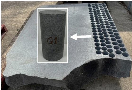
Figure 2. Slab of Adelaide black granite and a representative prepared specimen.
