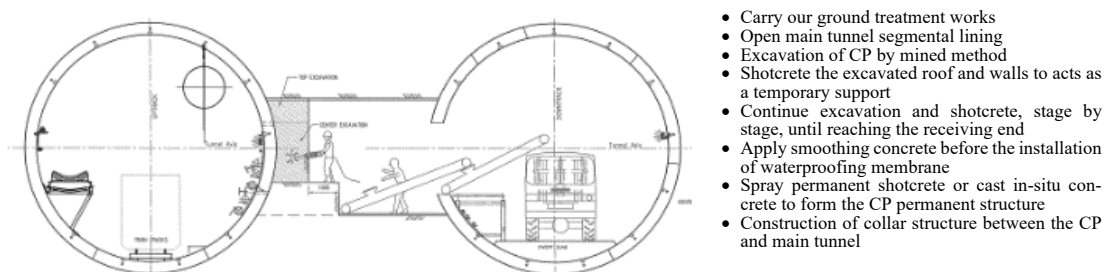
Figure 1. Typical construction of cross passage.
