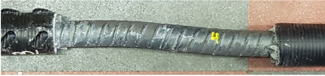
Figure 6. An example of a bolt, taken at the shear plane, following loading to 20mm shear displacement test.
