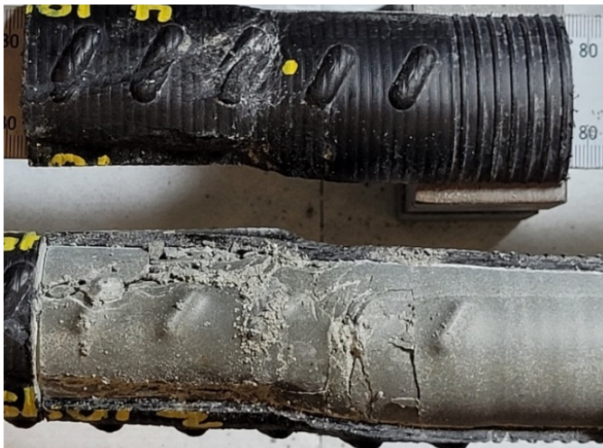
Figure 4. Sectioning of a tested CT26WR bolt sample at the shear plane, following 20mm of shear displacement. The inner annulus of cement grout has substantively held together during deformation of the bolt at the shear plane.
