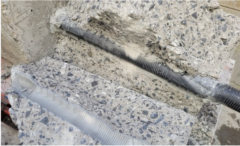
Figure 3. Initial sectioning of a CT26WR shear test sample after 20mm of shear. The centre block has been halved and opened, with the outer grout annulus remaining intact (lower left section), also revealing the bolt and sheathing (upper right section).
