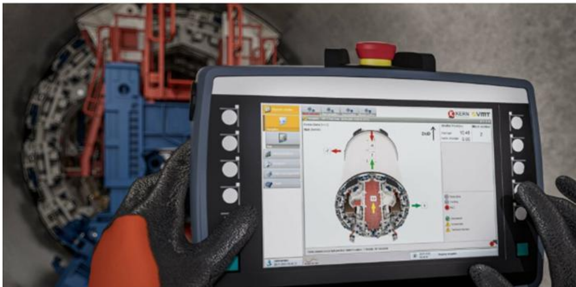
Figure 3. Positioning main screen from operators view during setup phase of a shutter
