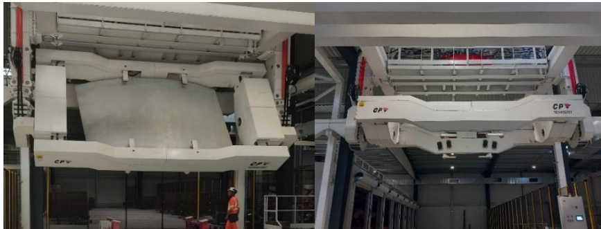
(a) Device holding a concrete segment. (b) Empty device with exposed contact pads.
