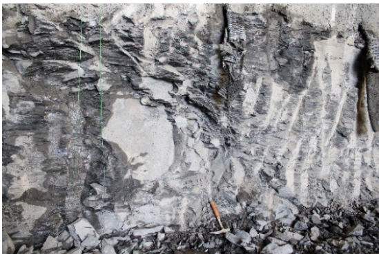
Figure 3. Fresh Ashfield Shale (Class II to Class I) with typical defects
