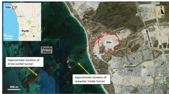
Figure 1. Plan layout of Outfall and Intake Tunnel.
