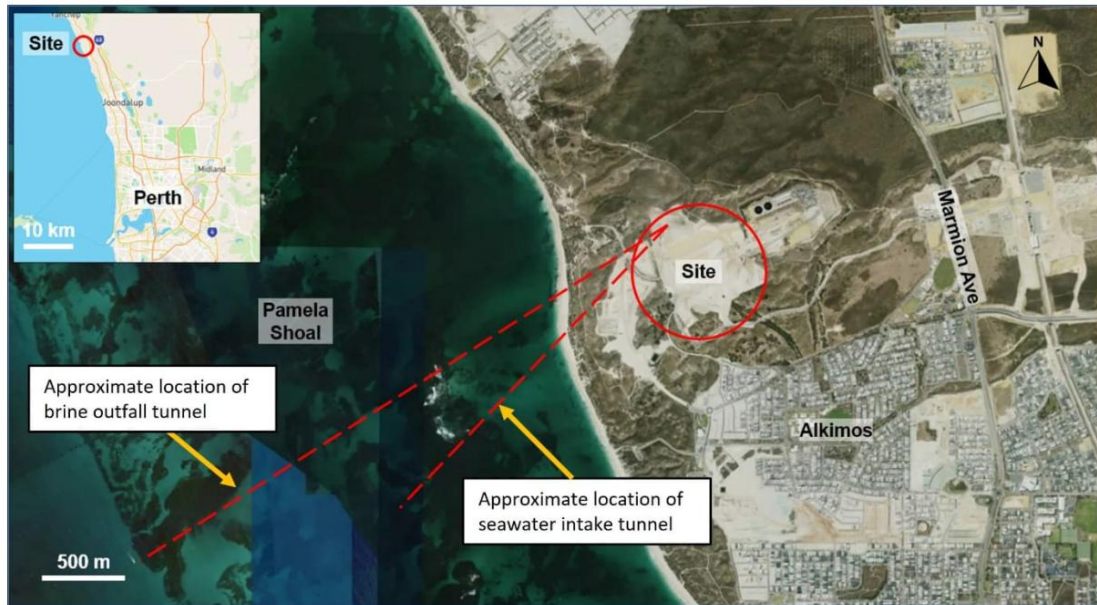
Figure 1 Plan layout of Outfall and Intake Tunnel
