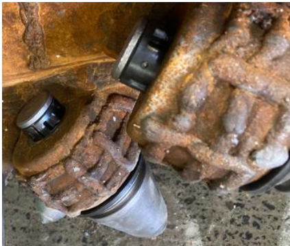
Figure 11. FLRRH picks installed in Mitsui Roadheader drum
