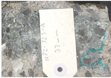
Figure 6. High water penetration result impacted by sample preparation and presence of aggregate.
