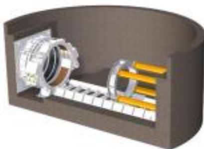
Figure 7. Pipe brake with launch seal installed in the launch shaft.
