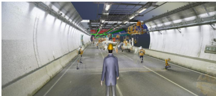
Figure 4. Point cloud survey overlaying the 3D model.
