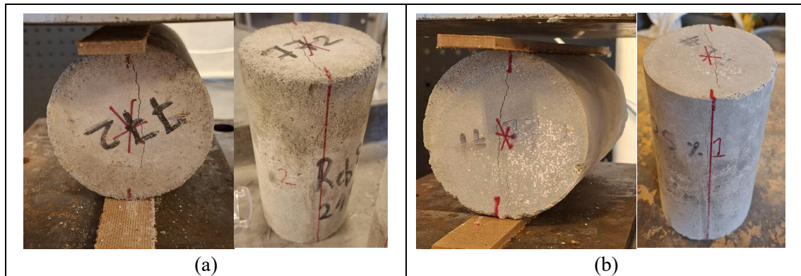
Figure 6. Brazilian test samples for (a) reference and (b) 25% replacement mix.
