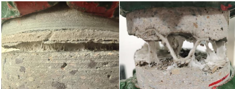
Figure 7. The failure state of the interface layer
