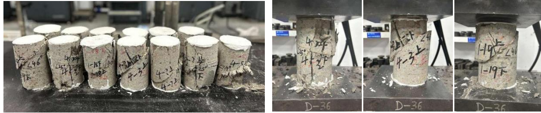
(a) Destructive specimens after testing (b) The failure state of specimens at different angles Figure 3. The failure state of the test specimen in the interface layer shear test
