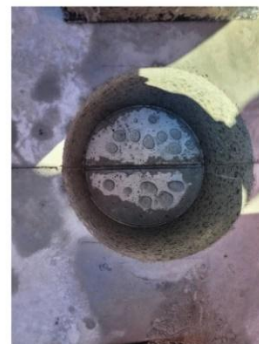
e) Segment coring test - bottom of core hole without damage
