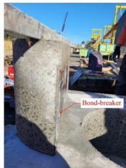
d) Half-circle core easily removed with bond-breaker attached
