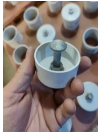
Figure 4. Threaded bolt centralized in casting lid
