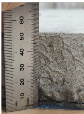
Figure 12: appr. 50mm thick mortar layer on membrane
