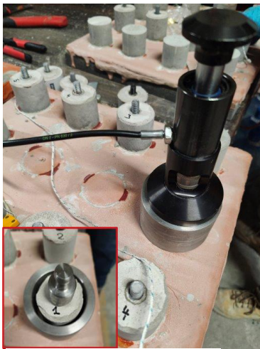
Figure 6: Load Application System
