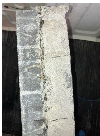
Figure 20: Sandwich specimen after heating at 160°C
