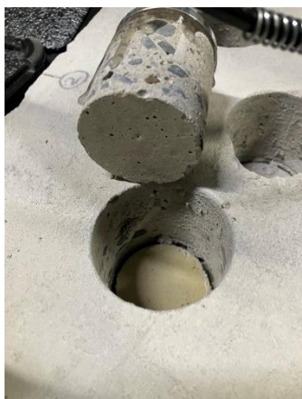
Figure 19: Pull off test – adhesion failure to secondary lining
