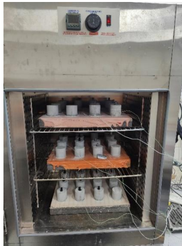
Figure 7. Sample slabs inside the oven
