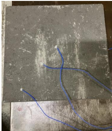
Figure 9: Thermocouple 1, 2 and 3 placed from corner to center of paver
