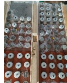
Figure 5. Cylindrical specimens cast and covered for curing
