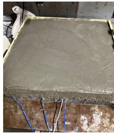
Figure 11: Sprayed membrane sandwiched between concrete paver and cement mortar layer
