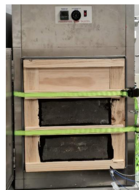
Figure 15: specimen placed for heat exposure
