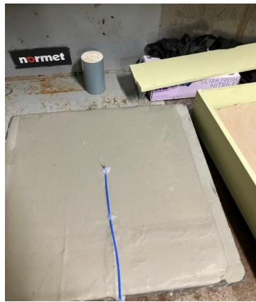
Figure 10: Thermocouple 4 elevated and placed in center of mortar layer
