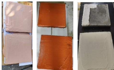
Figures 2a, 2b and 2c. Concrete Pavers coated with 3mm thick membranes 1, 2 and 3.
