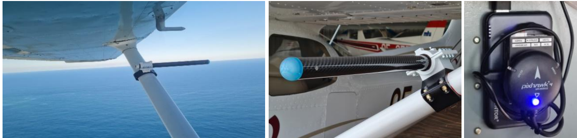
Figure 2. Self-contained flow sensor probe mounted on the strut (left and middle picture) and inertial sensors mounted in the cockpit (right picture)
