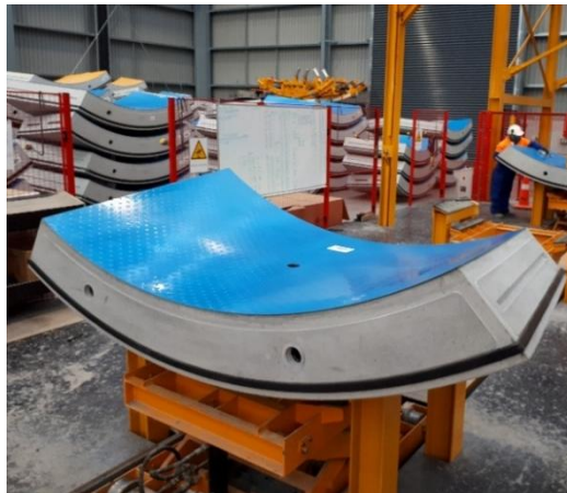
Figure 3. Tunnel PE corrosion protection liner segment in precast facility.
