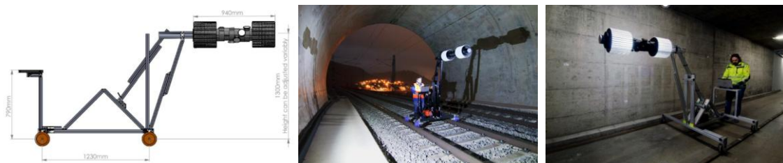
Figure 3. Vehicle-mounted tunnel scanning system equipped with laser profiler and DSLR cameras for 360° image and geometry capture.
