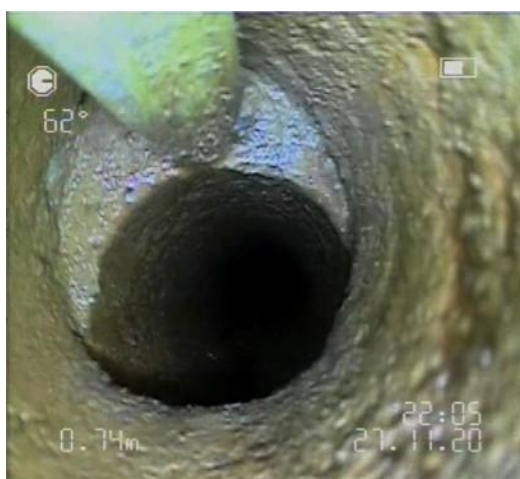
Figure 11: Uphole view of sheared bedding parting in endoscope hole. A rod of known dimension is placed against the shearing plane to assess the shearing magnitude (17 mm in this case). Source: Bai et al (2023).
